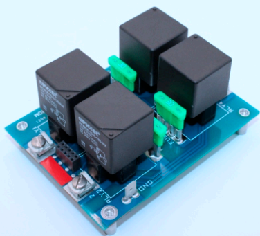
Replacement relay board for 4000 Series Control Modules
