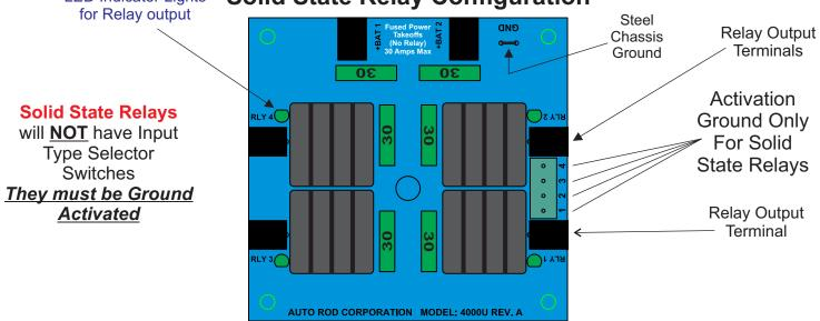
Solid State Relay use has to be configured at time of purchase SS Relays can only be used where they are assigned at ARC.
