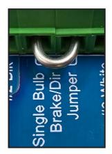
Separate bulb taillights use a separate bulb for turn signals and a separate bulb for brake lamps. *Remove* the silver jumper for separate bulb taillights. The light green wires will go to the brake lamp bulbs and the green and yellow wires will go to the directional bulbs.
